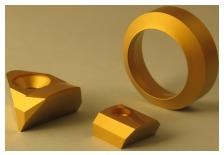
DIMOTEK FEATURES THE COMPLETE LINE OF HARD METAL RINGS FOR INTERNAL SCARFING WHICH ARE AVAILABLE IN 42° (GENERAL PURPOSE) AND 48° (ALLUMINAZED TUBES), IN DIFFERENT GRADES, PVD OR CVD COATED, OR WITHOUT ANY COATING.
