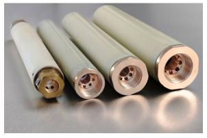
IMPEDERS DRAMATICALLY IMPROVE THE EFFICIENCY OF THE WELDING PROCESS BY DIRECTING MORE ENERGY TOWARDS THE EDGES OF THE STRIP. AN IMPEDER IS SIMPLY ONE OR MORE FERRITE CORES CONTAINED WITHIN A SUITABLE NON-METALLIC HOUSING.
